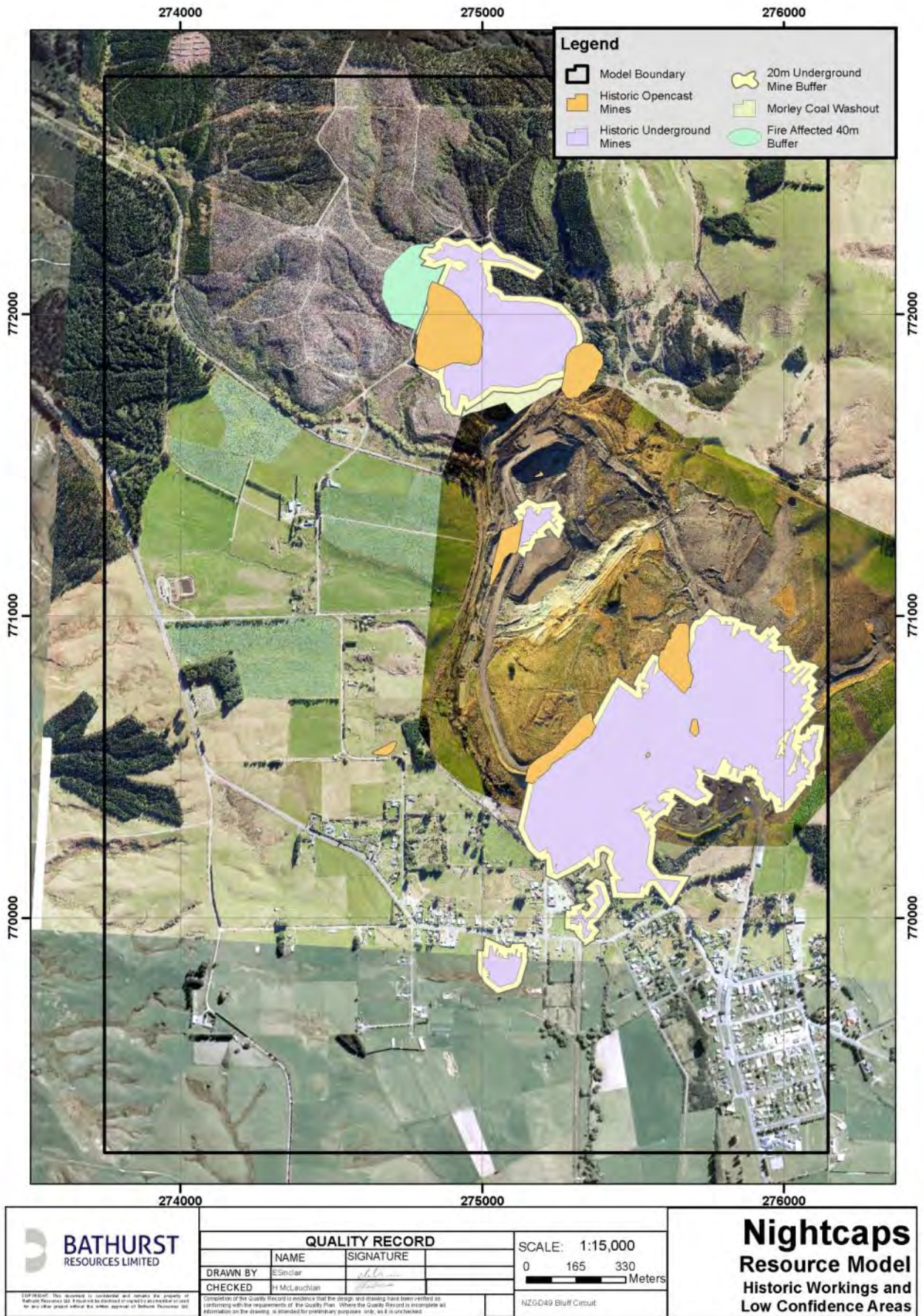
Figure 13 Location of historic mine workings and areas of low confidence. Note: Recent opencast mined areas are not shown. Extent of Coaldale pit is shown by aerial photo from end June 2016.
