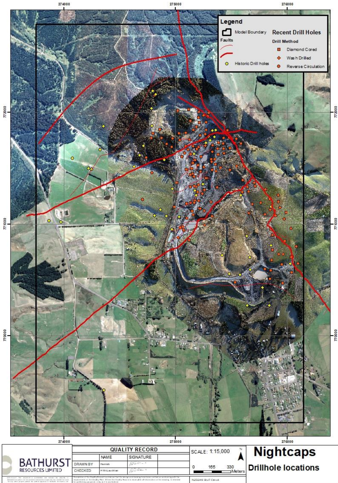
Figure 12: Location of drilling and major faults within Resource Area
