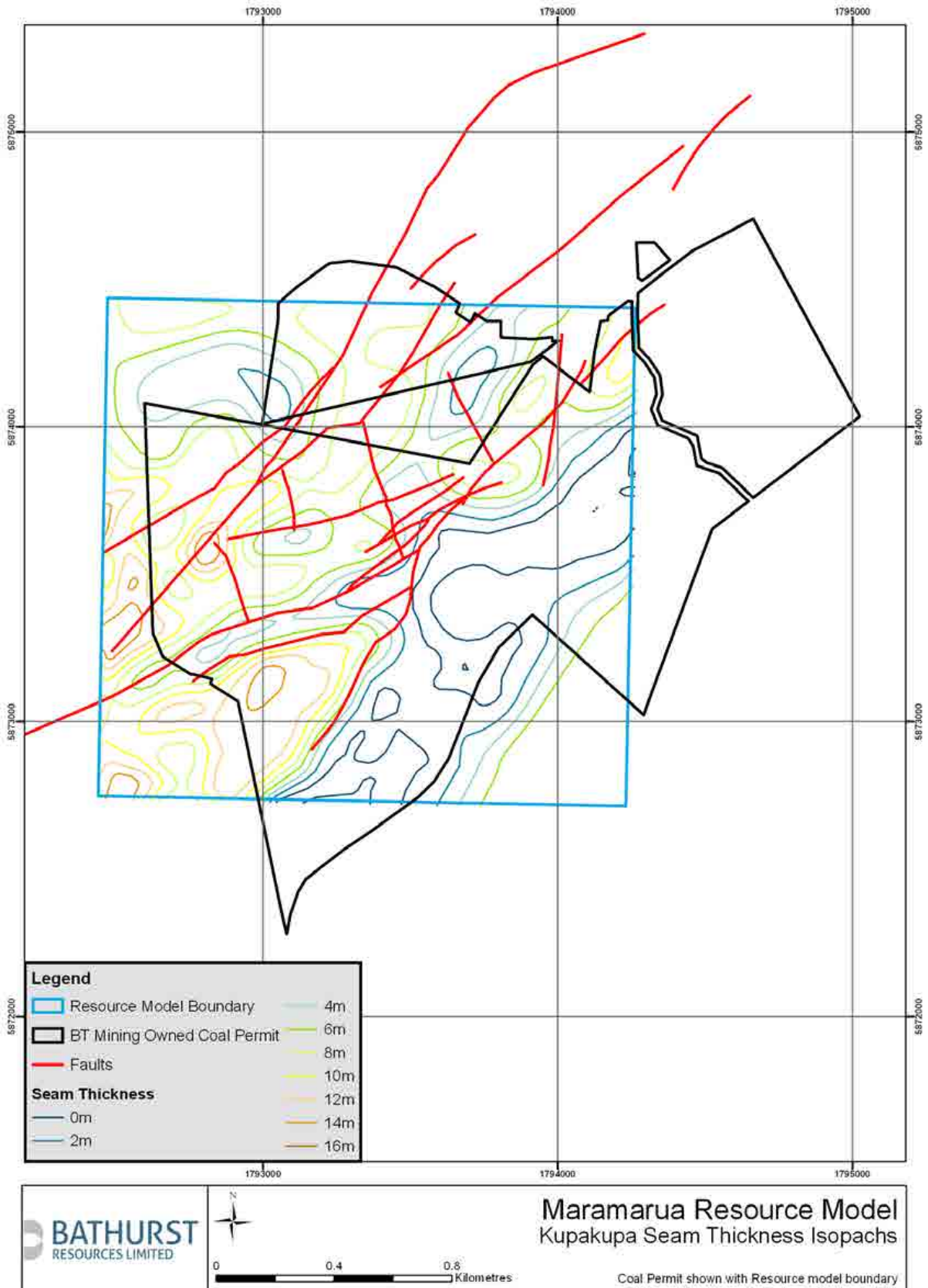
Figure 7: Plan showing full seam thickness contours over the model area
