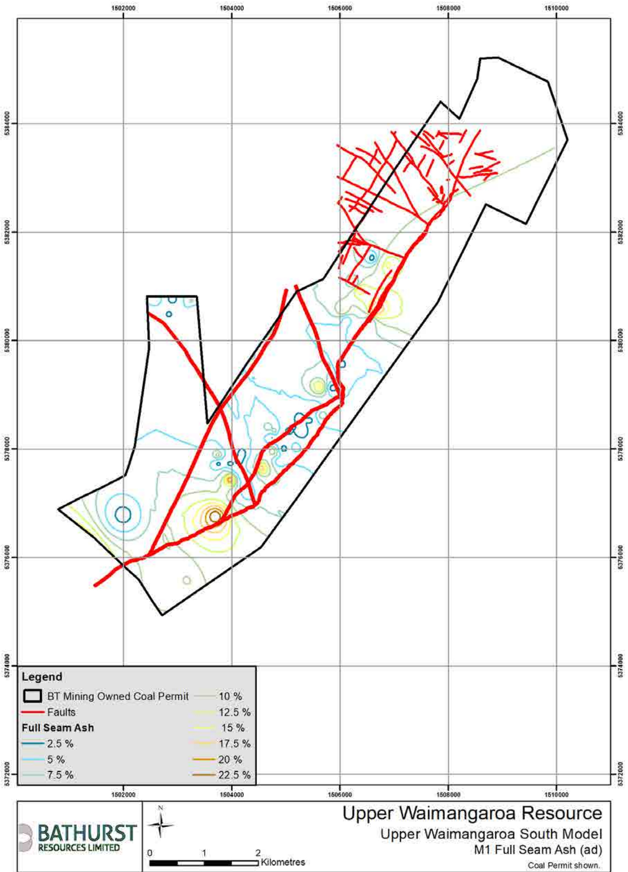
Figure 11 Plan showing in-situ full M1 seam ash on an air dried basis across the Upper Waimangaroa South resource
