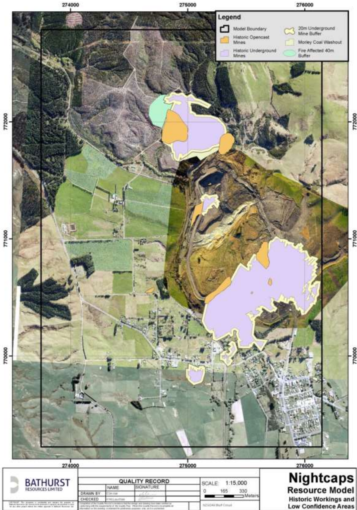
Figure 13: Location of historic mine workings and areas of low confidence. Note: Recent opencast mined areas are not shown.
