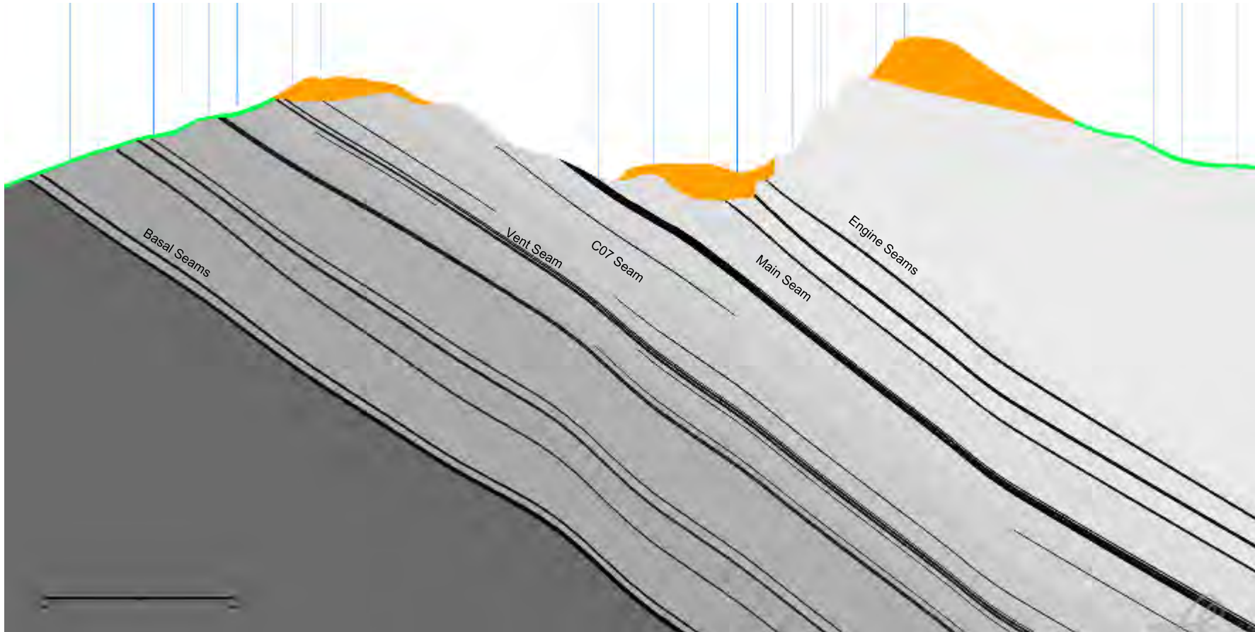
Figure 9: North west facing section through the working seam section at Canterbury Opencast Mine
