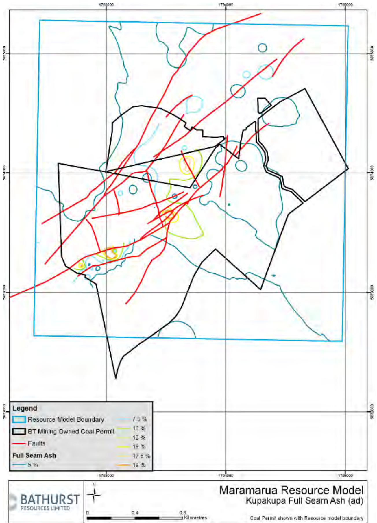
Figure 8: Plan showing in situ full seam ash on an air-dried basis as modelled over the deposit area
