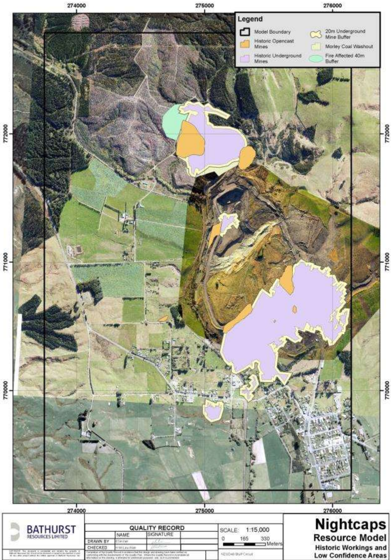
Figure 39 Location of historic mine workings and areas of low confidence. Note: Recent opencast mined areas are not shown
